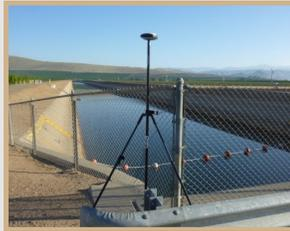
A GPS/GNSS receiver collecting data at an elevation monitoring station
